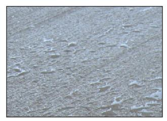
Water is applied over AQUA-GUARD 3 hours after initial application. This broom finished concrete surface demonstrates the early water resistance properties that develop with the AQUA-GUARD sealer.
